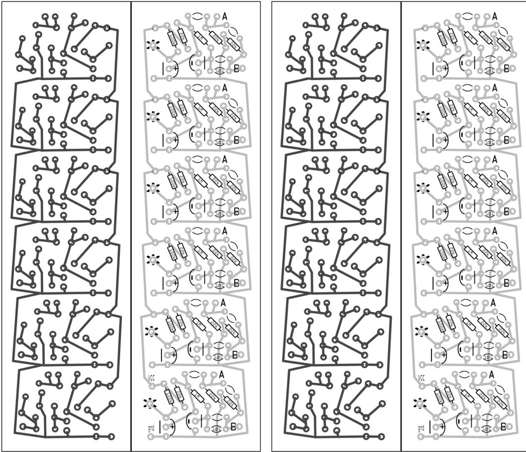
These were made with 2n3904 and 2n3906 transistors in mind... Most transistors should work, but mind the orientation. BC556, BC546, and other transistors would need flipped, so check before you solder. I also omitted one sandrode, because I found it unnecessary, it would be connected to the base of the  $NPN$ .
